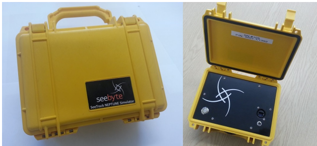
Fig. 3. The Neptune simulator used during MIRIAM development. It simulates either one or two AUVs running the Neptune Autonomy Framework (Figure 7). Configuration files allow simulation of factors including the onset of various faults and accelerated battery drain due to adverse environment conditions.
