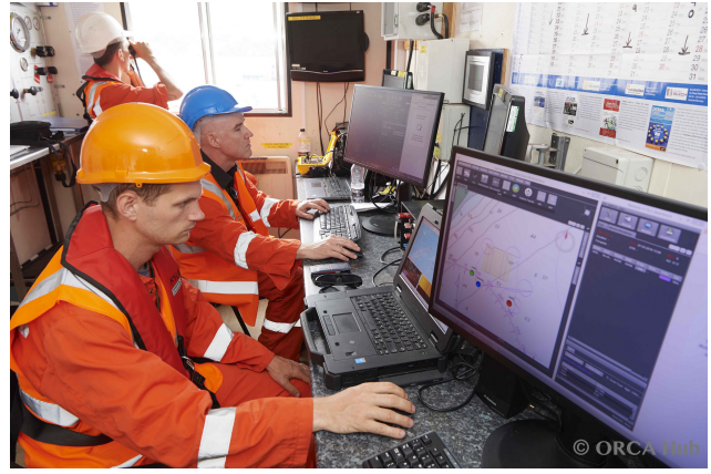
Fig. 9. On-shore control room. An operator controls the communications relay Sonobot USV separately using dedicated software. While the IVER-3 AUV mission can be monitored on the SeeTrack/Neptune/MIRIAM interfaces.
