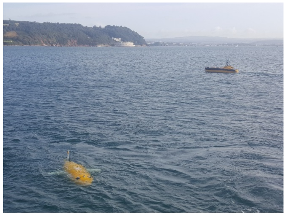
Fig. 1: Example of cooperative mission between a surface and subsurface vehicle. ASV's C-Worker is equipped with an USBL to support NOC's Autosub Long Range performing a survey.
