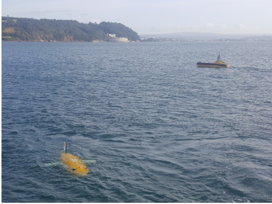
Fig. 65: Cooperative mission between C-Worker 5 (equipped with engines which forces it to drive continuously at a minimum speed) and Autosub Long Range (a slow moving vehicle at roughly 0.5 knots).
