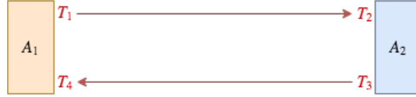
Fig. 8: A message exchange between platform A_1 and A_2 can be used to synchronise A_1 's clock in respect to A_2 or for A_1 to measure distance between them.
